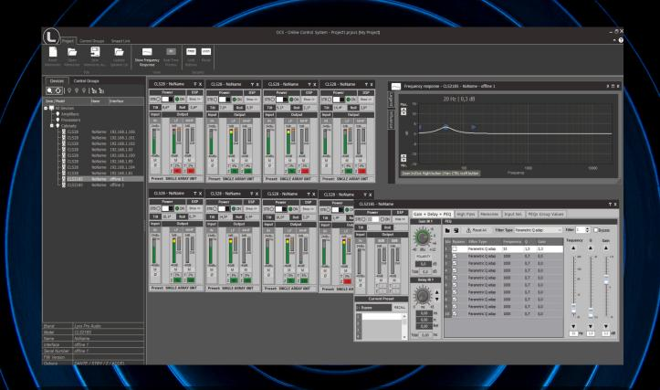
OCS is our control and monitoring software, working in real time for all our digital processing systems (cabinets, processors and amplifiers). It is a user interface enabling the set-up of all digital devices in an installation, allowing control via Ethernet / USB (one device).
