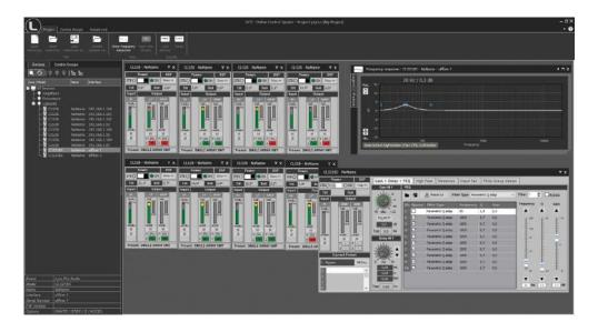
Control and monitoring software for multiple devices (loudspeakers, amplifiers and processors). Allows control via Ethernet / USB for Lynx Pro Audio systems with integrated DSP.
