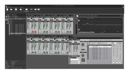
Control and monitoring software for multiple devices (loudspeakers, amplifiers and processors). Allows control via Ethernet / USB for Lynx Pro Audio systems with integrated DSP.
