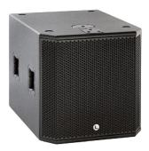
The lonic-18S is a powered subwoofer enclosure part of the lonic series. It uses  $1 \times 18$ " (3" voice coil) neodymium transducers offering an ultra compact subwoofer enclosure with 132dB SPL. The power module (Class D with switching power supply) includes a DSP which offers different presets to cover a wide range of sound applications complementing the column speakers. Ionic-18S provides quick and easy set ups for both fixed installations and portable applications.
