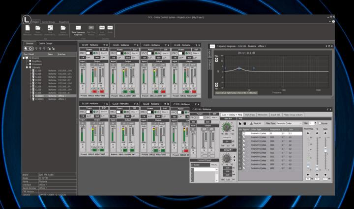
OCS is our control and monitoring software, working in real time for all our digital processing systems (cabinets, processors and amplifiers). It is a user interface enabling the set-up of all digital devices in an installation, allowing control via Ethernet / USB (one device).
