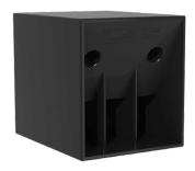
The DS-18S is an extremelly high power subwoofer cabinet providing exceptional low frequency reinforcement for the DS-12. It uses one 18" (4" DUO voice coil) transducer with aluminium demodulating ring in direct radiation bass reflex configuration. Manufactured as standard with premium birch plywood and finished with polyurea coating it can also be manufactured in any colour or finish to compliment any install design.
