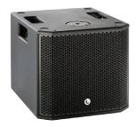
The lonic-12S is a powered subwoofer enclosure part of the lonic series. It uses  $1 \times 12$ " (3" voice coil) neodymium transducers offering an ultra compact subwoofer enclosure with 127dB SPL. The power module (Class D with switching power supply) includes a DSP which offers different presets to cover a wide range of sound applications complementing the column speakers. Ionic-12S provides quick and easy set ups for both fixed installations and portable applications.
