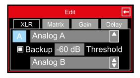
This screen allows you to configure your XLR input. You can select the desired input channel and choose between Analog mode and setting a Threshold level.
