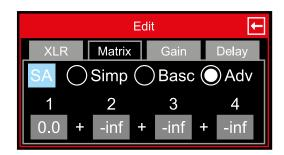
The edit screen allows you to adjust advanced Matrix configuration options. You can then configure the matrix with more specific parameters.
